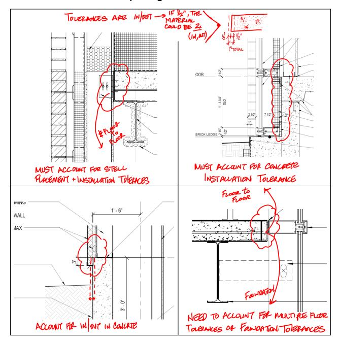
New construction or renovation...both need proper construction tolerance.
